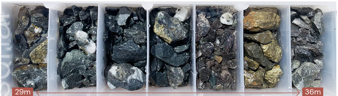
Figure 1. WNR0017; 7.0m (5.6m*) @ 3.58% Cu and 3.96 g/t Au from 29.0m including 2.0m (1.6m*) @ 10.23% Cu and 13.62g/t Au from 34.0m.
