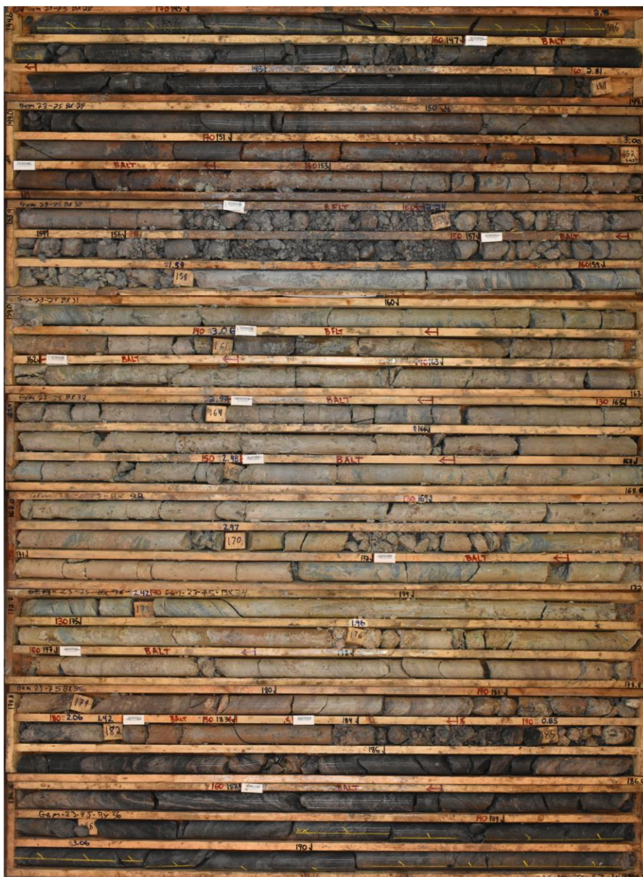
Figure 2: Strong brittle faulting with intense hydrothermal alteration in GEM23-075
