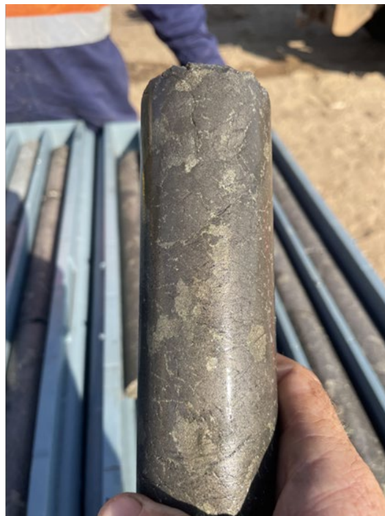
Figure 1: 23WKDD003 at 179.1 m - massive sulphide mineralisation with visually logged Ni and Cu sulphides (refer to BUX ASX announcement 4th October 2023).
