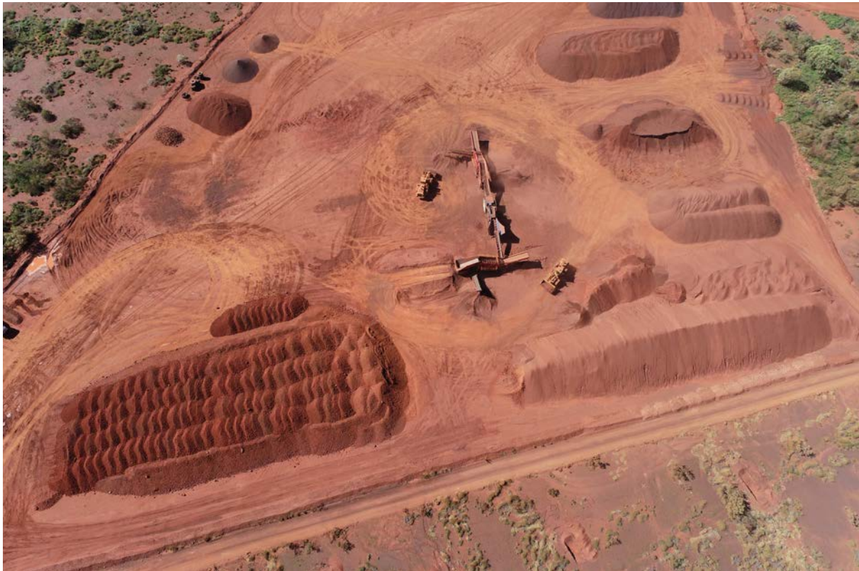
Figure 2: Detritals mining operations – crushing unit and stockpiles, June 2022
