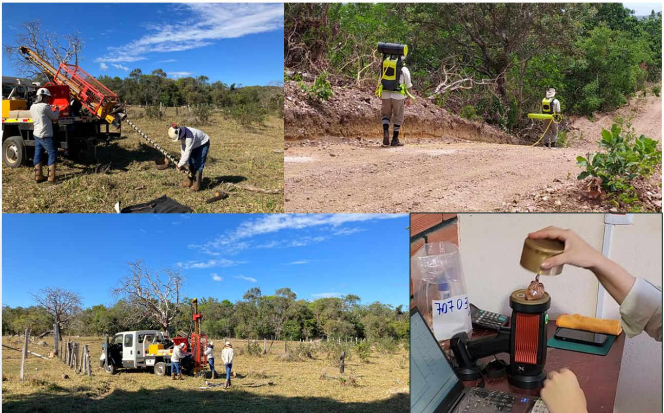
Figure 4: Alvo's auger rig drilling at Bluebush REE Project (Boa Vista Prospect top and bottom left). Loupe Electromagnetic equipment in action at Boa Vista (top right) and SciApps X-555 portable XRF analyzer in action at Alvo's core shed (bottom right).
