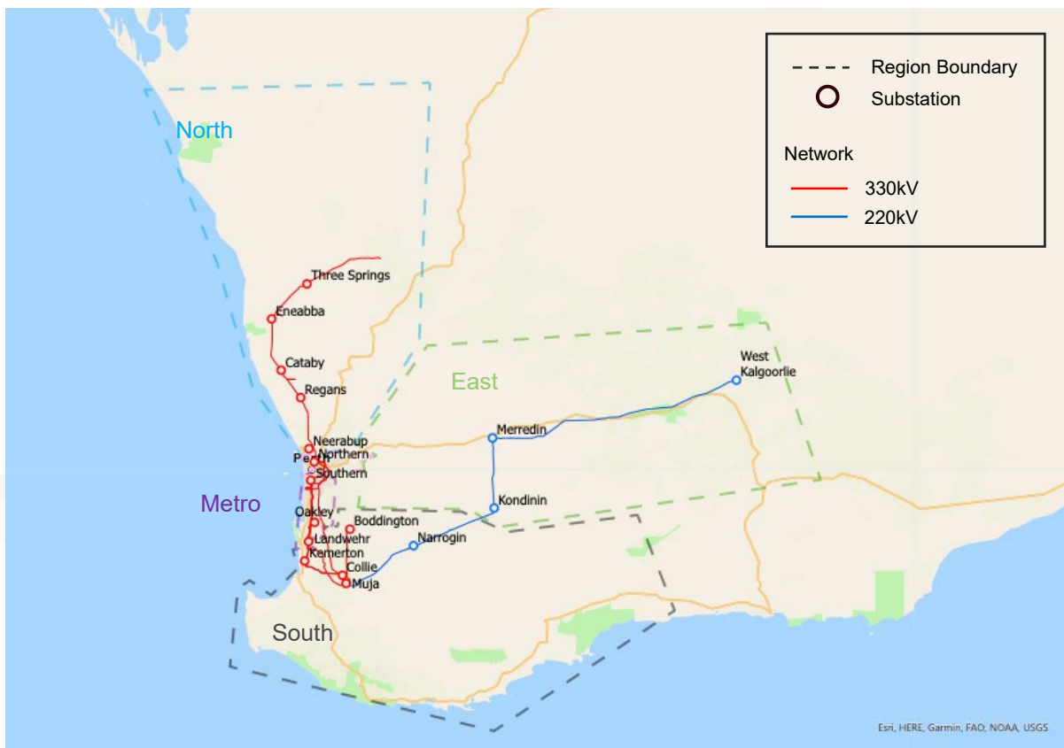
Figure 1 SWIS 330kV – 220kV network and Regions
