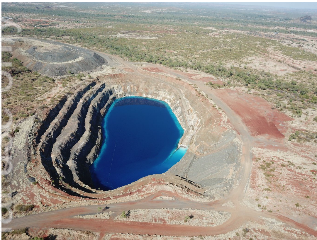
Figure 4. Great Australia Mine with Advanced Grade Control drilling areas cleared to the east (proposed cutback area) prior to dewatering activities.
