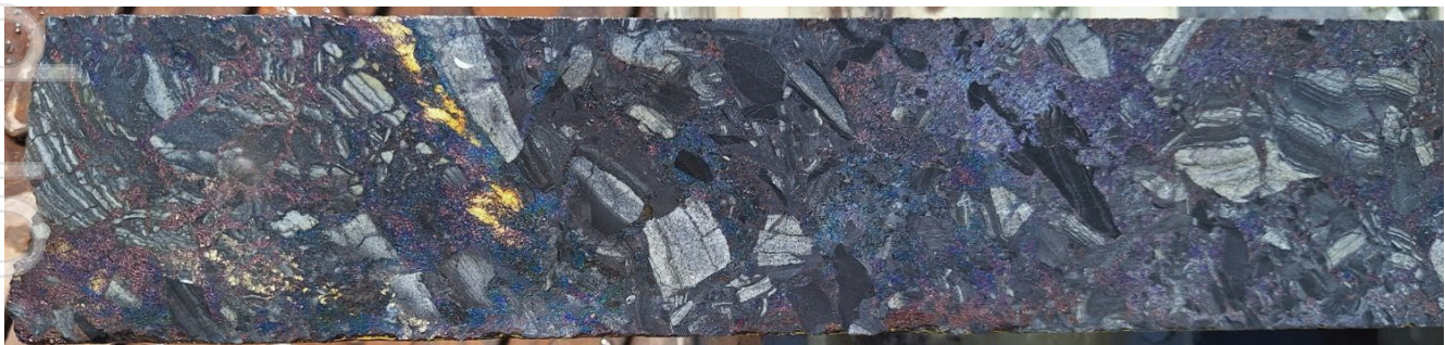
Figure 8. High-grade chalcocite, covellite, bornite & chalcopyrite sulphide matrix breccia in the upper intercept MOXD 217-1.10 m @ 24.8% Cu, 93.2 g/t Ag and 1,125 ppm Co from within the 66.50m (48.00m*) @ 4.95% Cu, 32.7 g/t Ag and 686ppm Co from 234.00m. 1
