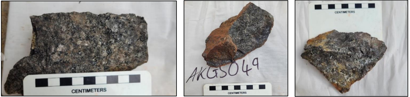
Figure 9. Rock chip samples of ultramafic intrusive rocks at the Arkun project, WA. These rocks and prospects can potentially host nickel copper PGM deposits, and follow-up fieldwork is a priority.
