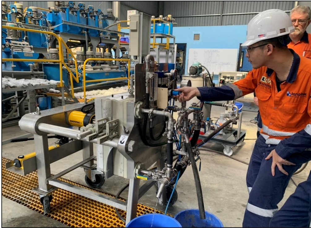
Figure 7 - Vendor piloting - Pressure filtration testwork trials
