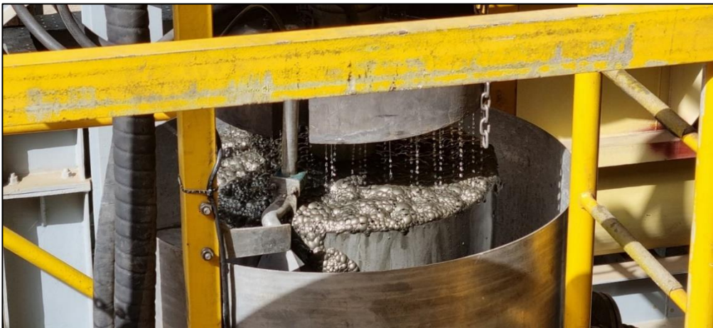
Figure 6: Vendor piloting - Jameson Cell trials producing improvements in Nickel and MgO concentrate grades.
