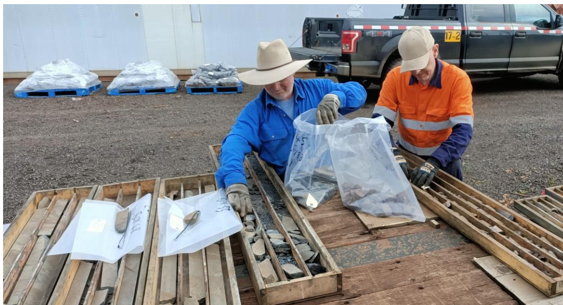
Image 3 - Drill cores were selected and packaged for shipping to metallurgical laboratory.
