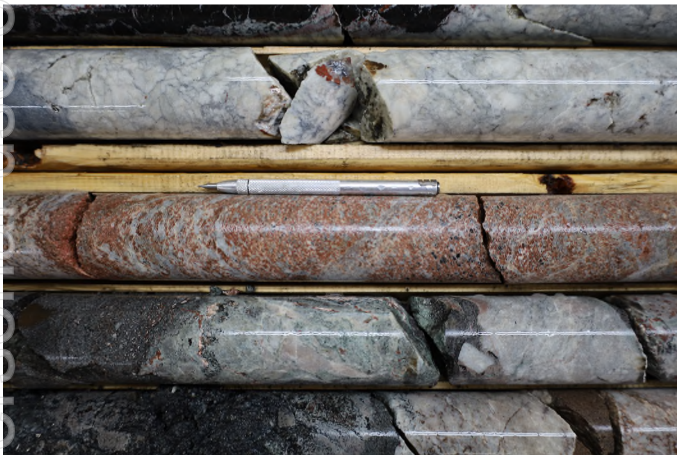
Figure 4: Diamond drill core (NQ, approximately 4.8 cm diameter) containing strong REE mineralisation (red coloured disseminations to semi-massive) within ferrocarbonatite/calcioarbonatite host rock. Hole POM-23-03, 173m downhole depth.
