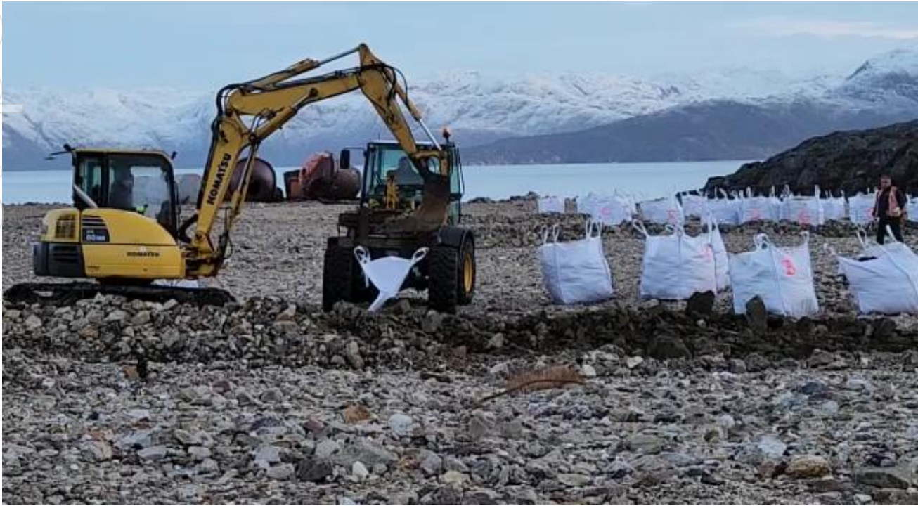
Figure 80: Collecting several tonnes of bulk samples from 5 trenches in the mineralized dumps
