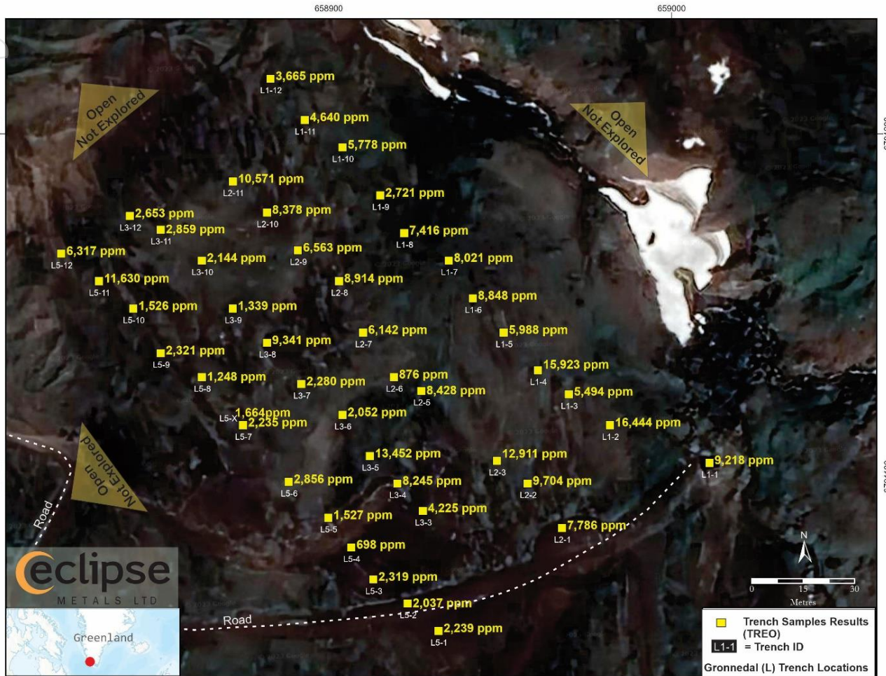
Figure 1: Grønnedal trench sample results in the lower section with REO mineralisation in all trenches. Note that, to date, only a small fraction of this prospect has been explored and that the system is open in all directions
