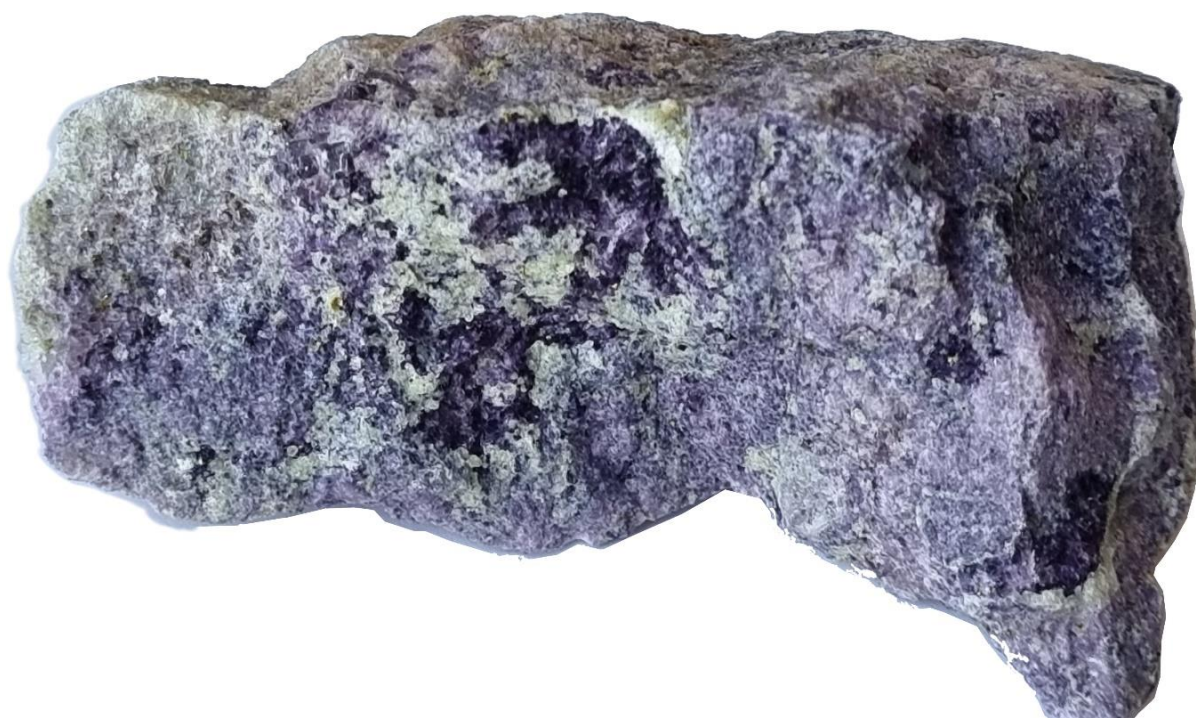
Figure 124: Mineralised waste dump specimen visually estimate to consist of 70% Purple Fluorite; 25% Green Fluorite; and 5% Cryolite.
