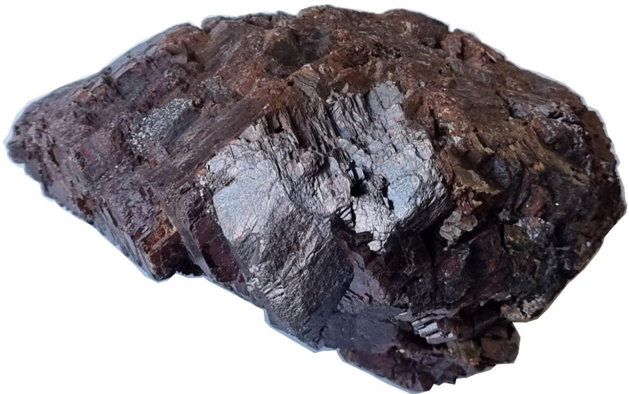
Figure 113: Mineralised waste dump specimen visually estimated to consist of 90% siderite and 10% cryolite.
