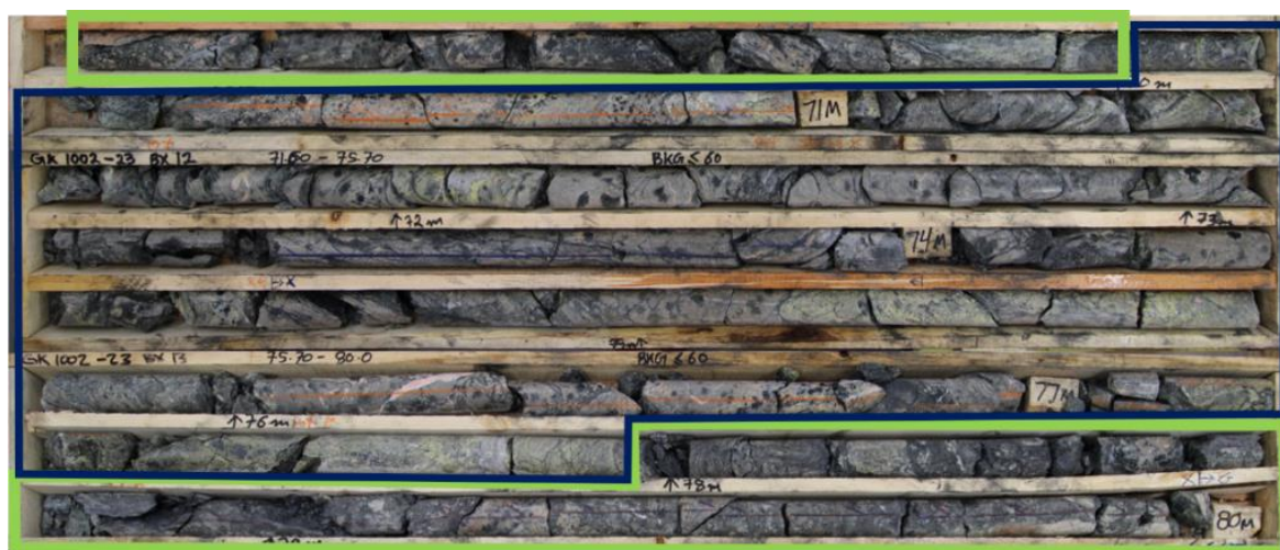
Figure 6: Faulted interval in drillhole GKI-002 characterised by successive moderately to strongly chloritized and argillised cataclastic fault cores (green box) separated by a damage zone (blue box)
