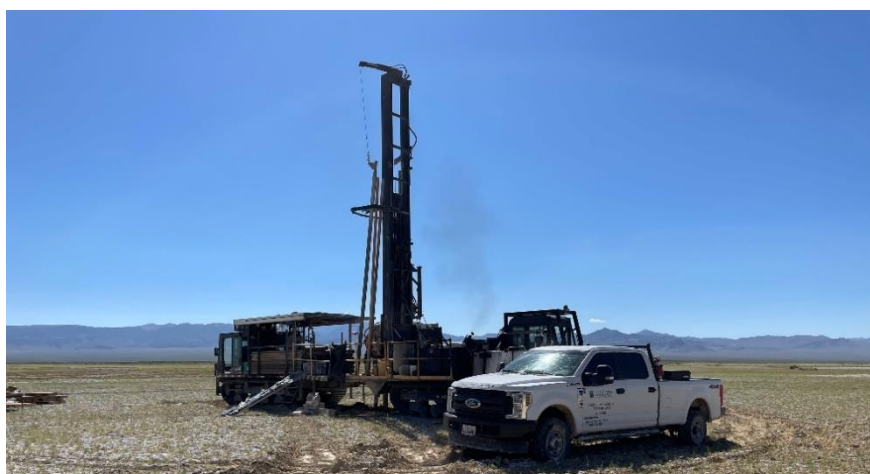
Figure 12: Sonic rig drilling at NBS Carvers
