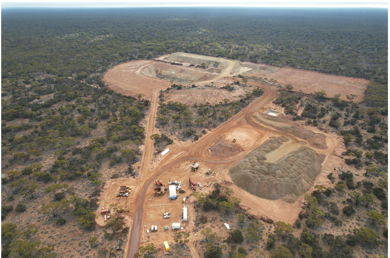
Figure 1. Jeffreys Find Mine Site at completion of the stage 1 pit – note Run of Mine ore stockpiles lower right.
