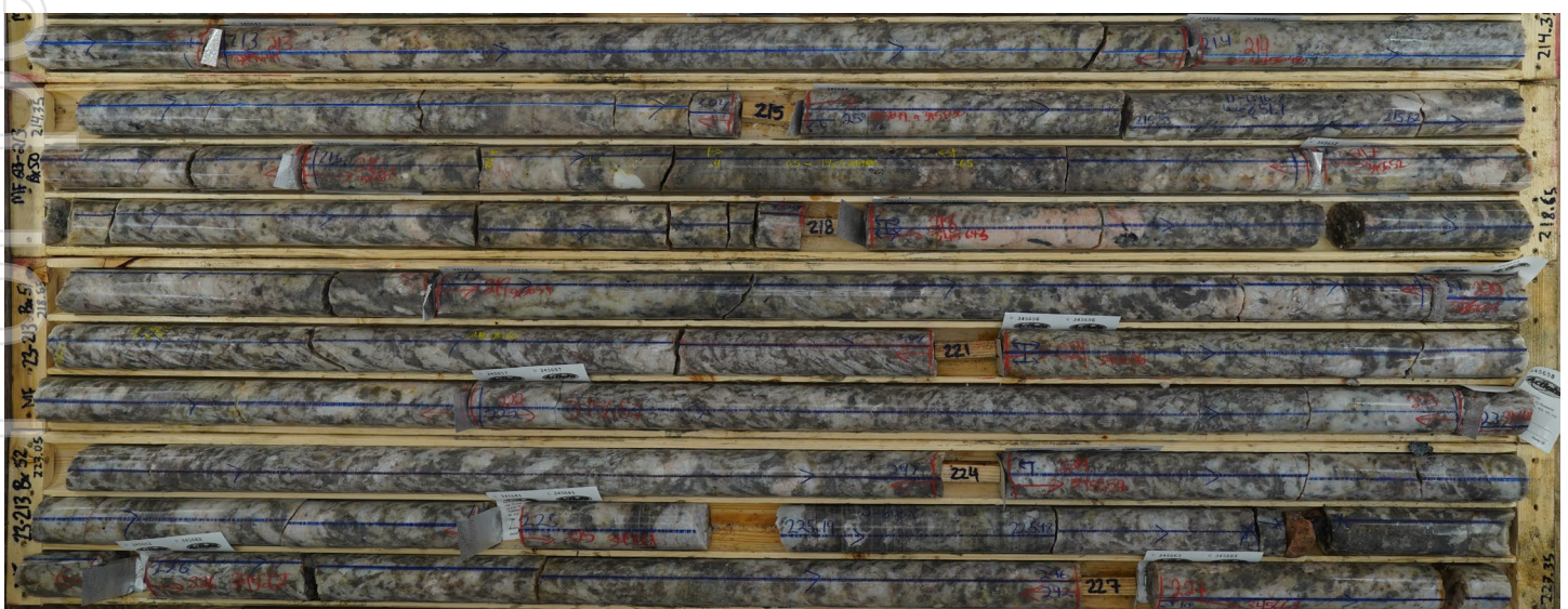
Figure 1 – A sample of drill core from drill-hole MF23-213 – high-grade, coarse-grain spodumene (from ~211m to ~227m down-hole)
