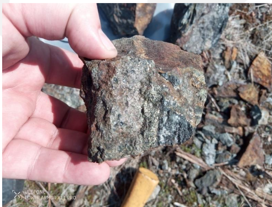
Figure 1 – Sample F0015010 – 3.48% Cu and >1% Ni – Semi-massive pyrite-pyrrhotite-pentlandite.
