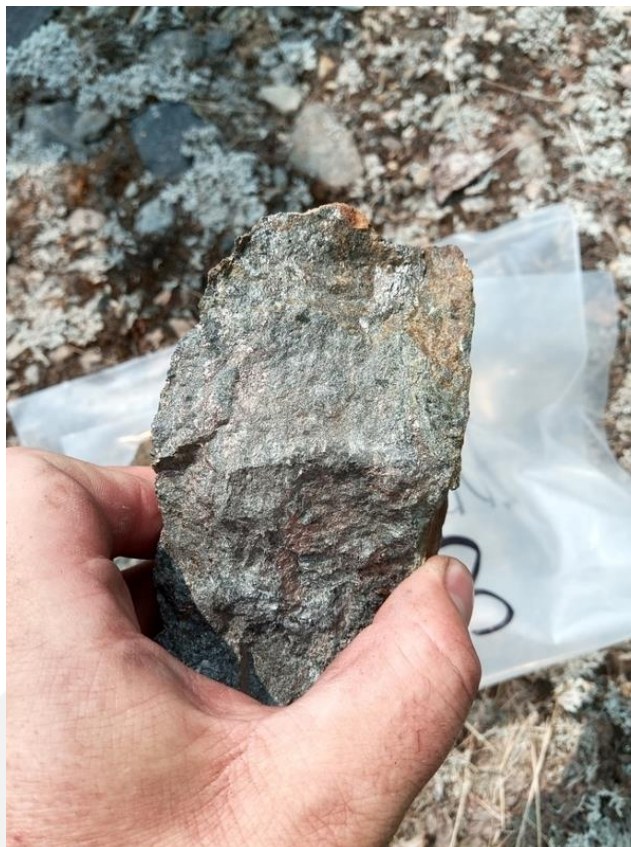
Figure 2 - Sample F0015073 - >1% Ni and 0.8% Cu – Chlorite-altered gabbro with pyrrhotite, pentlandite and chalcopyrite.
