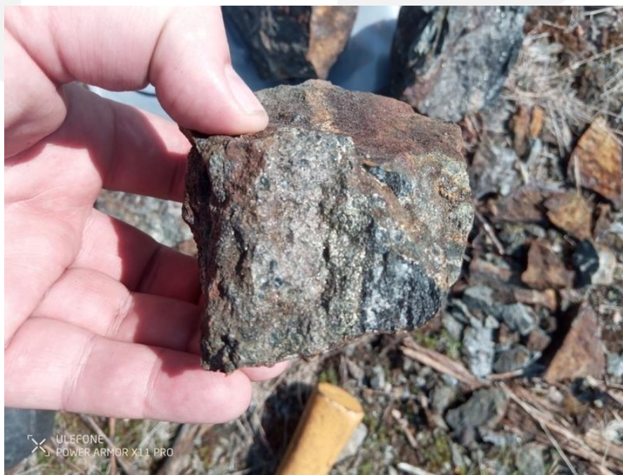
Figure 1 – Sample F0015010 – 3.48% Cu and >1% Ni – Semi-massive pyrite-pyrrhotite-pentlandite.
