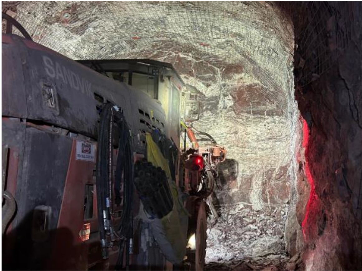
Figure 8 – Picture showing ore in a face underground in front of the Jumbo (photo 23 August 2023).
