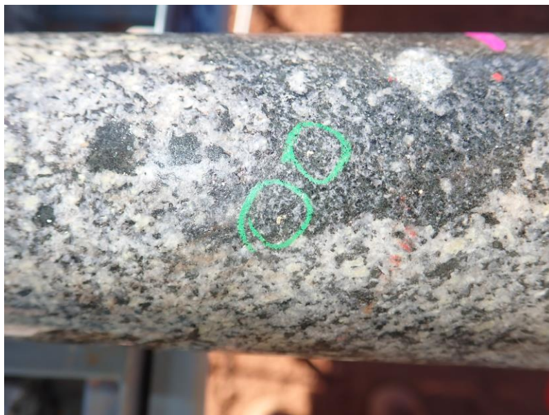
Figure 5. Example of chalcopyrite blebs associated with biotite-rich rafts in WSDD001 .
