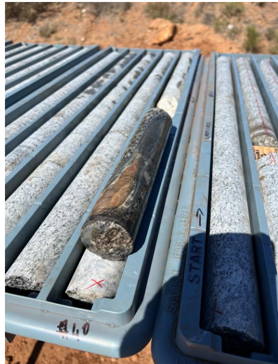
Figure 4. Chalcopyrite “seam” and iron oxide “raft” within narrow shear in biotite granodiorite (WSDD002 – 231.6m).
