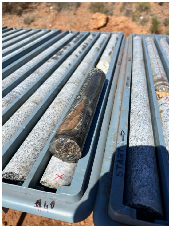
Figure 4. Chalcopyrite “seam” and iron oxide “raft” within narrow shear in biotite granodiorite (WSDD002 – 231.6m).
