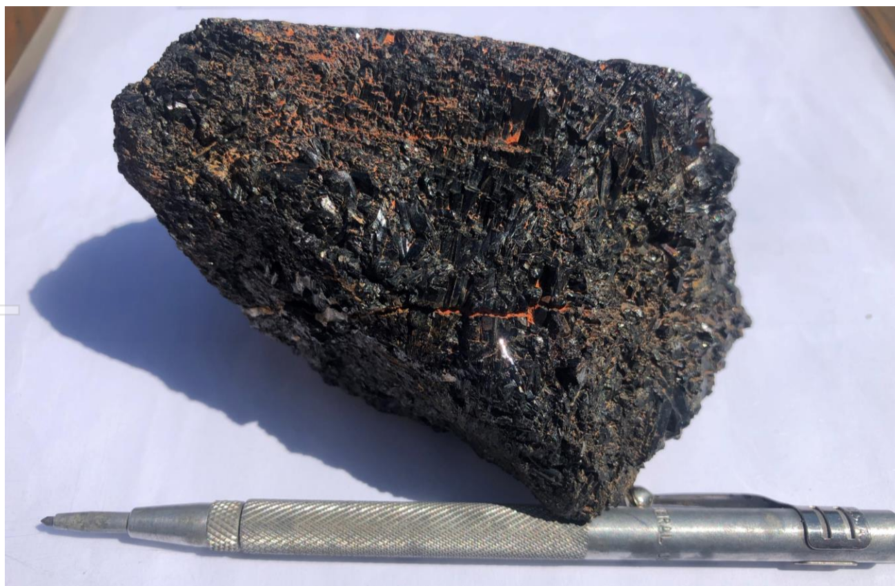
Figure 8: Fist sized cluster of black and amber coloured tourmaline in road cut at Itambacuri.
