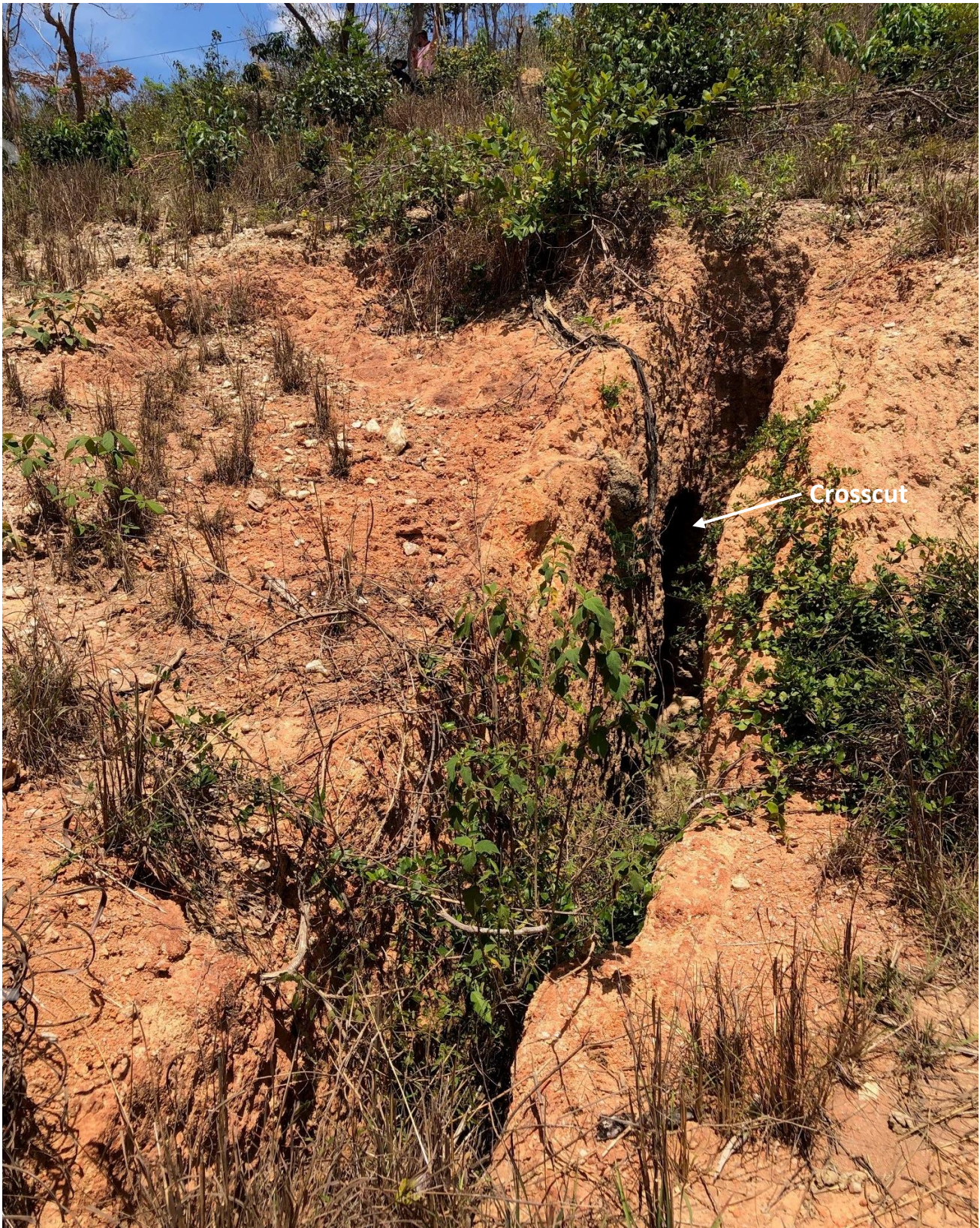
Figure 2: Carai artisanal mine workings for emeralds and green tourmaline. The workings consist of a 7m x 1m trench with crosscuts either side. There are also a number of shallow pits on the uphill side of the trench.
