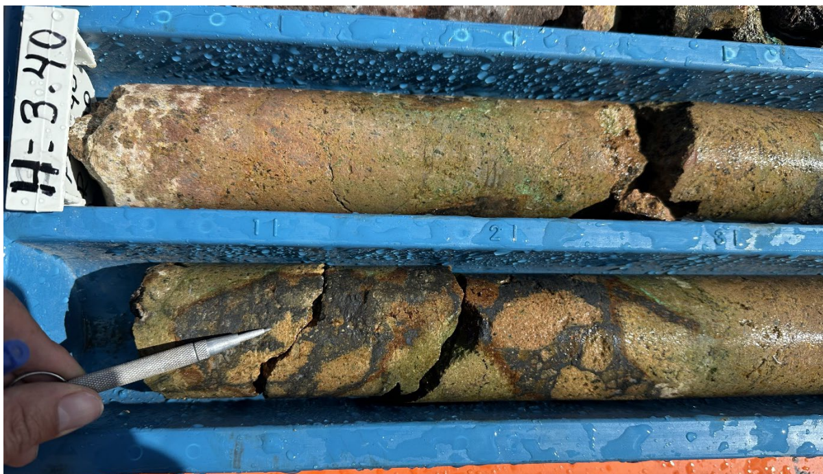
Figure 3: Example of secondary copper mineralisation at around 4.5m depth in 23PCMD0001
