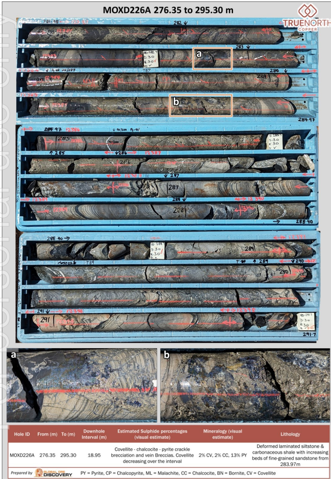
Figure 7. MOXD226A - 276.35m to 295.30m mineralisation example: chalcocite-covellite-pyrite crackle breccia (a) chalcocite-covellite-pyrite mosaic breccia (b).
