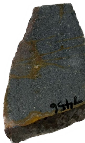
Figure 4. Sample 7456: 1.56g/t Au, 4.19g/t Ag, 249ppm As, 6.6ppm Sb and 55.5ppm Mo.
