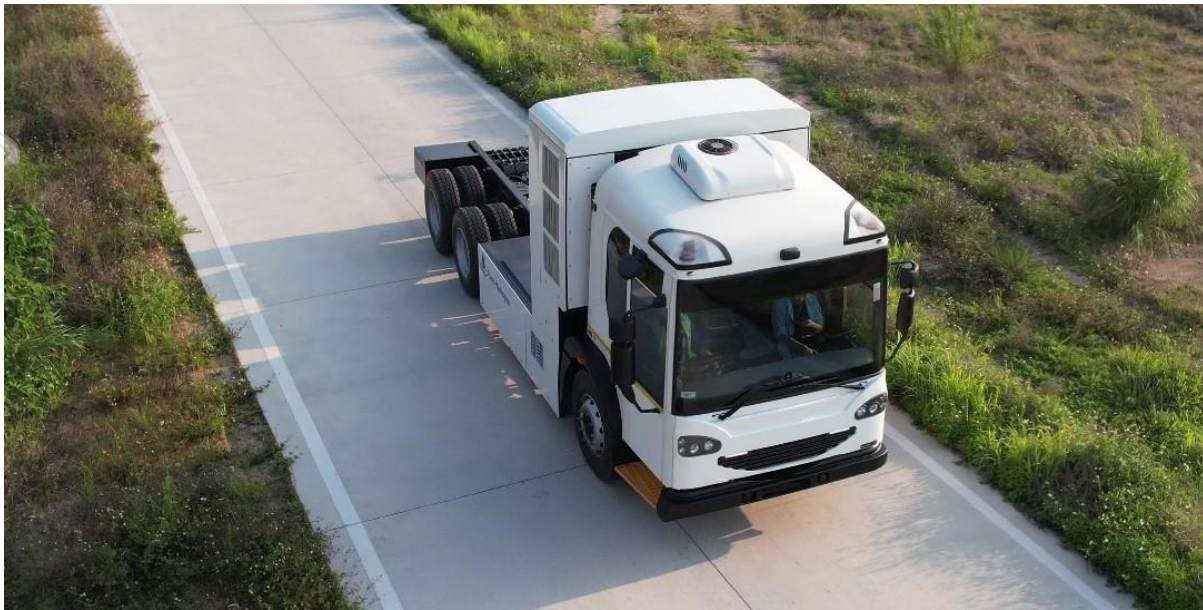
Image 2: Another view of Pure’s first hydrogen fuel cell waste collection vehicle.
