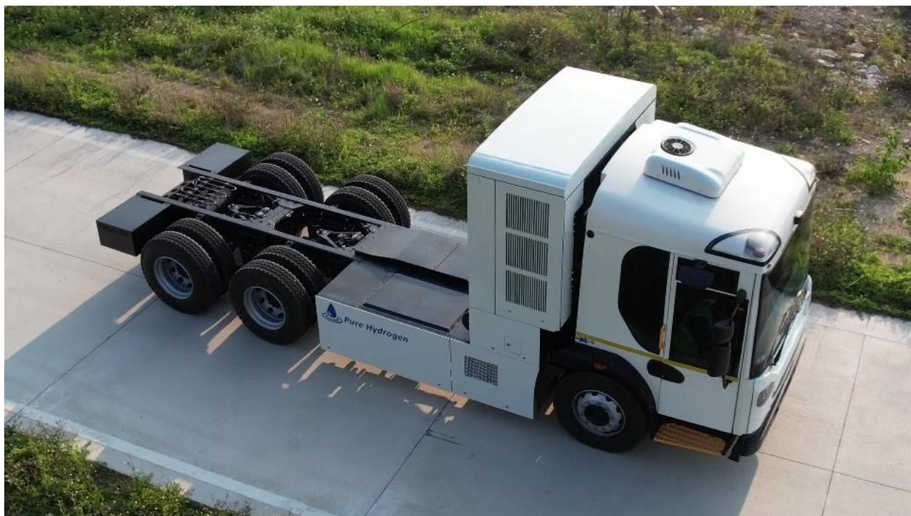
Image 1: An aerial image of Pure's first hydrogen fuel cell waste collection vehicle, which is now being fitted with refuse collection components by Bucher Municipal.
