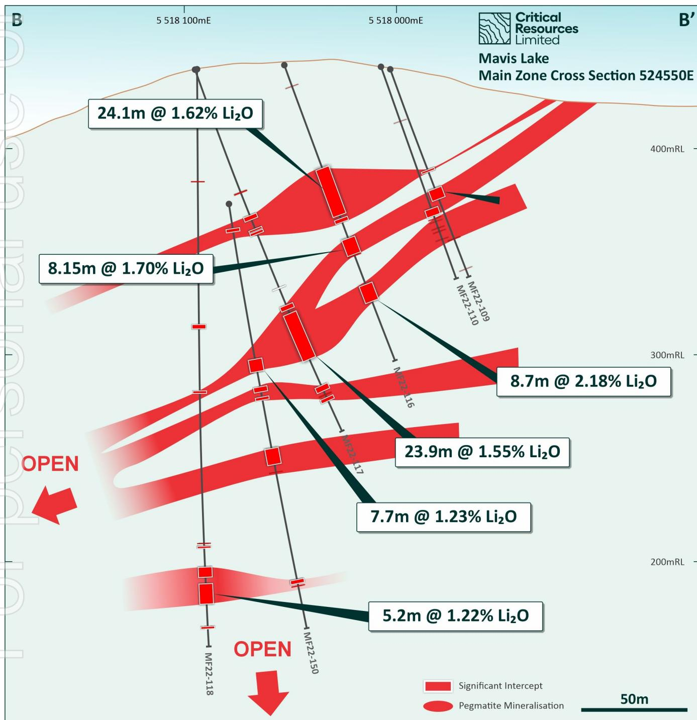
Figure 3: Section B-B' – Swell Zone near-surface
