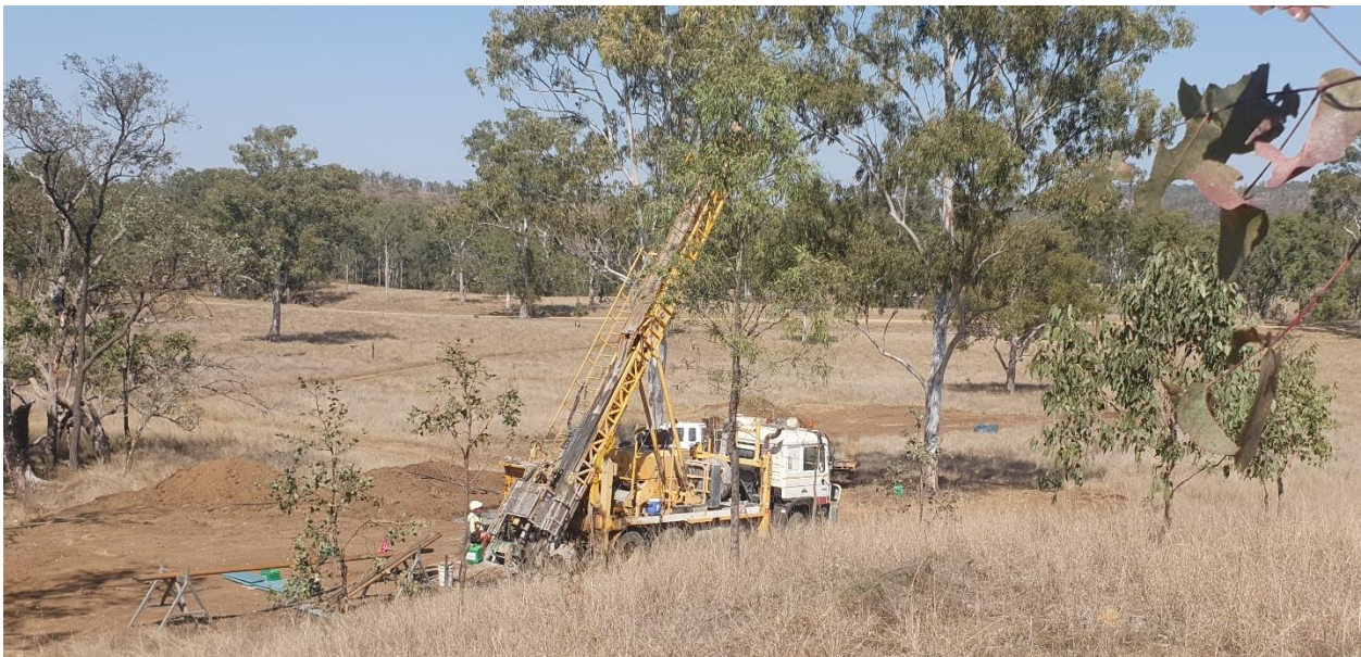
Figure 1: Diamond drilling in progress at the Yarrol Project's Central Ridge target
