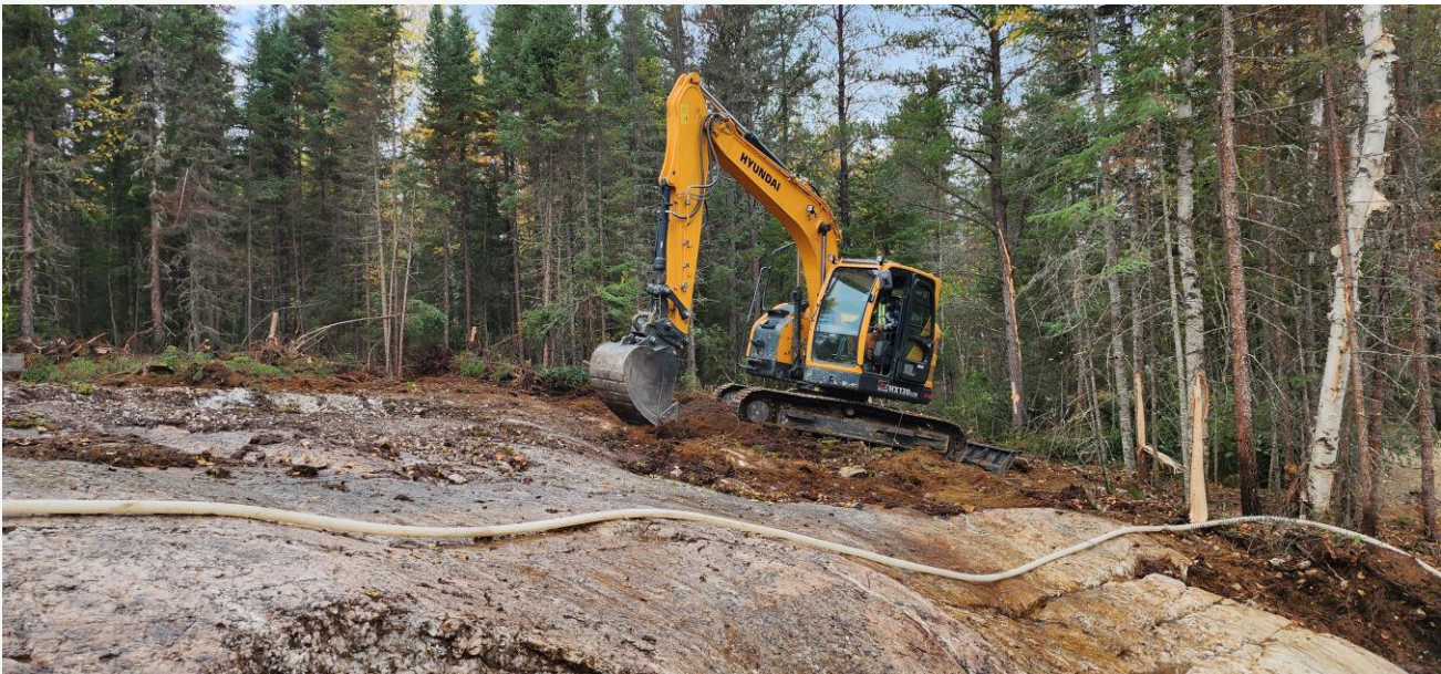
Figure 7 – Mechanical stripping of Koshman pegmatite
