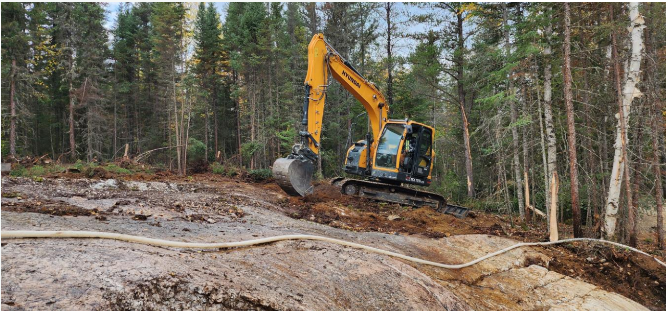
Figure 7 – Mechanical stripping of Koshman pegmatite
