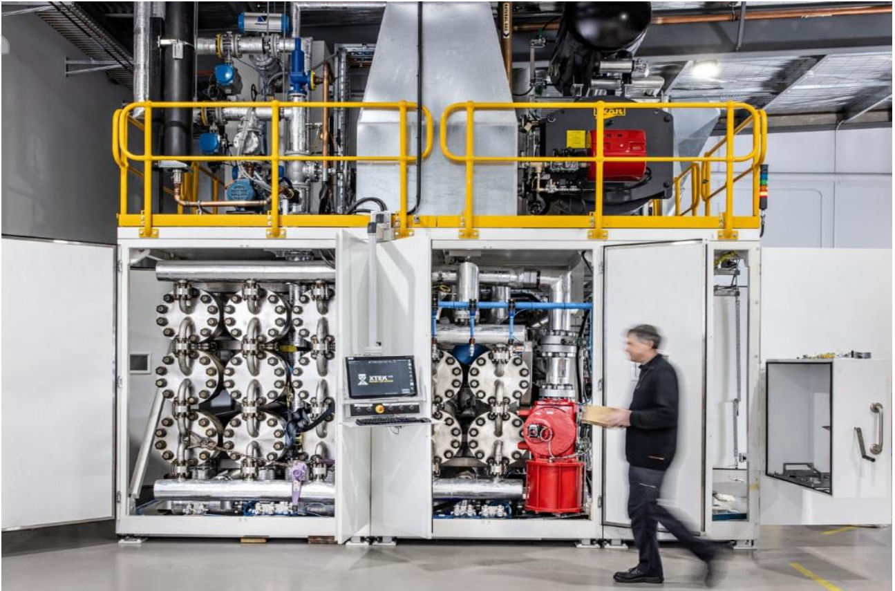
Image Above: XTEK's patented XTclave system operates at 200 degrees Celsius and 300 Bar of pressure, to make world leading, advanced ultra-lightweight and high-performance ballistic body armour and helmets.
