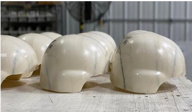
Image Above Left: Unpainted and unfurnished high-performance "rifle rated" advanced ballistic helmets, made in XTEK's patented XTclave system. Unlike "normal" helmets that only stop pistol bullets and fragmentation, these "Rifle Combat Helmets (RCH) stop AK-47 and other high-powered assault rifle and machine gun bullets.
