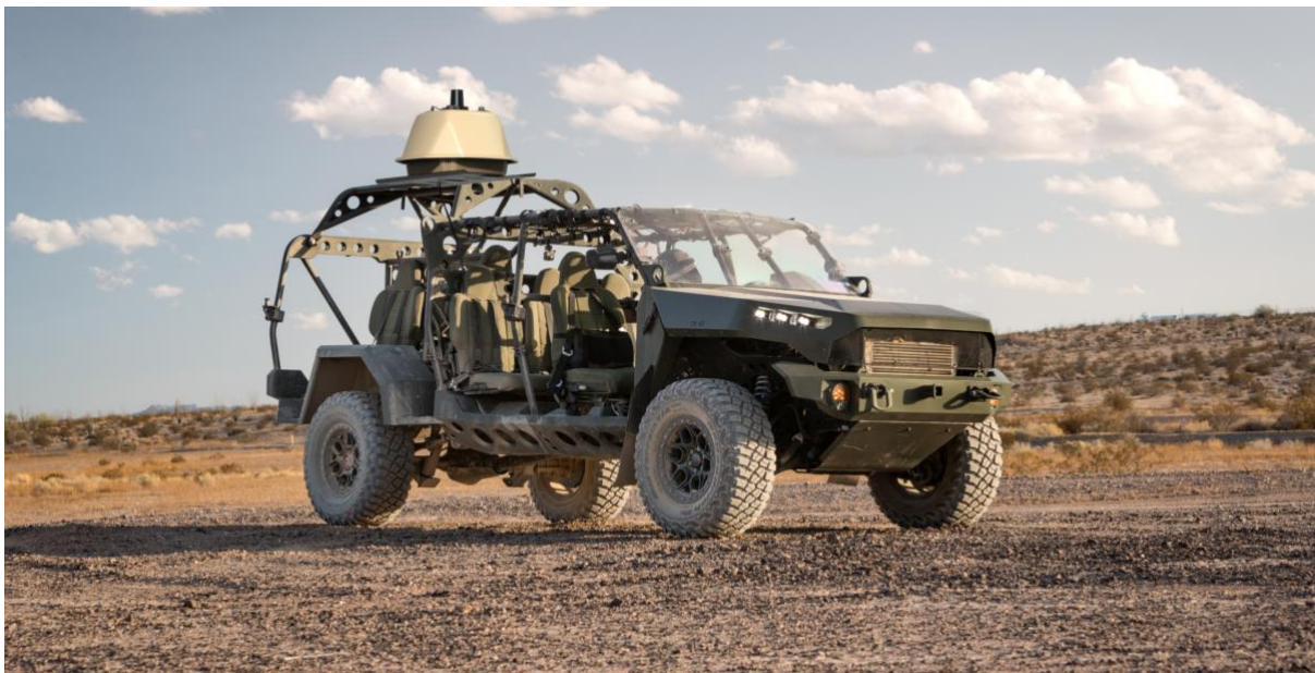
Image: DroneSentry-X Mk2™ mounted on a military squad vehicle
