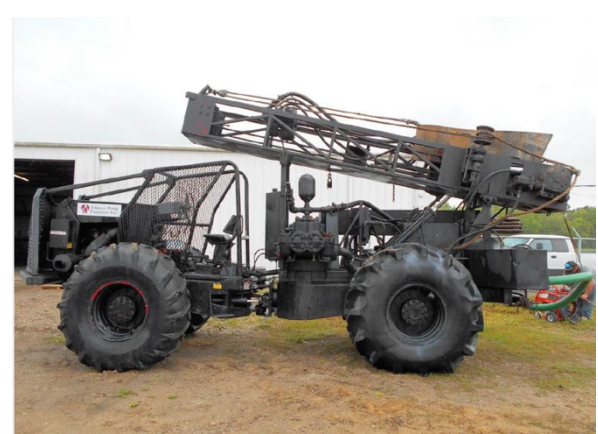
Figure 2: Soil test borehole drilling rig.
