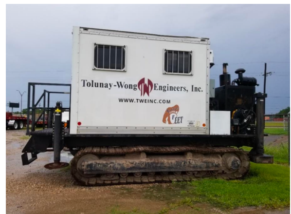
Figure 1: Cone penetration test (CPT) track mounted rig.
