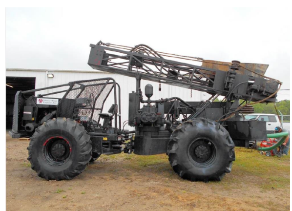
Figure 2: Soil test borehole drilling rig.
