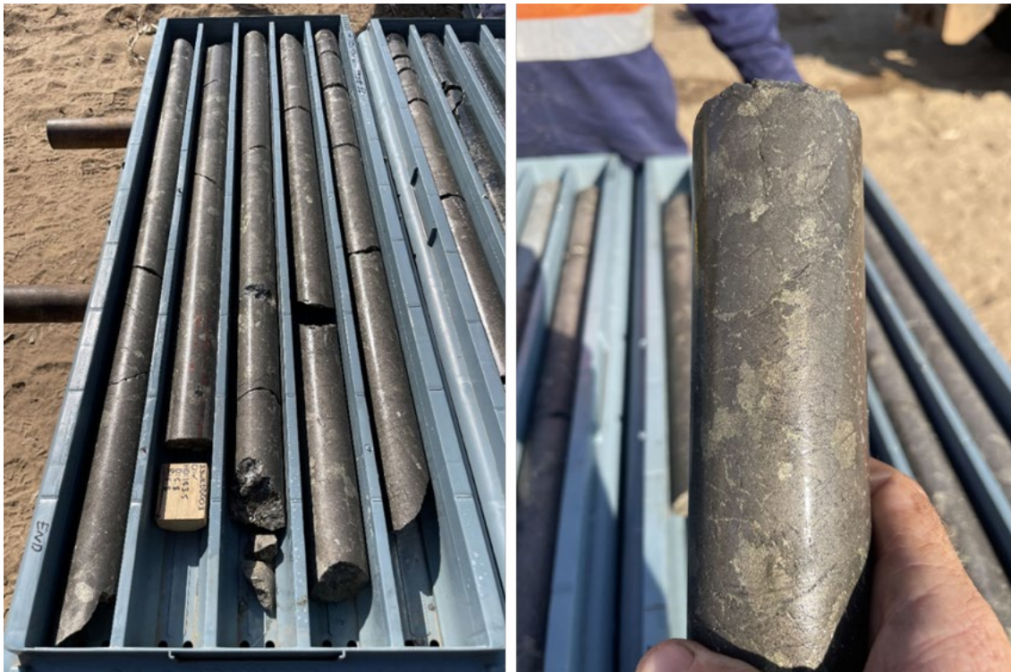
Figure 1: 23WKDD003 at 179.1 m - massive sulphide mineralisation with visually logged Ni and Cu sulphides.
