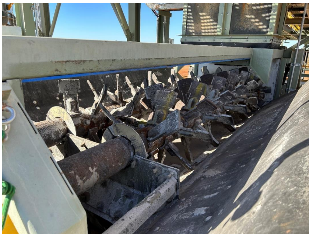
Figure 10 – Internal view of the paste mixer used for mixing paste (tailings and cement and water) at Abra (Photo 5 September 2023).
