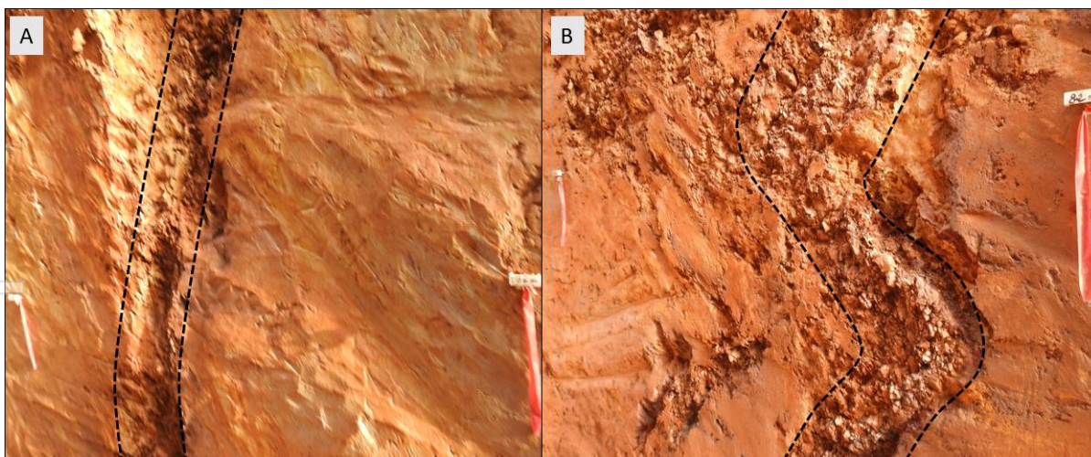
Figure 14: MSTR01 A) Steep north-west-plunging 20cm vuggy quartz vein at 74m, 36.4 g/t gold. B) 35cm wide, folded iron-rich vuggy quartz with disseminated sulphide from 82m, 4.7 g/t gold.
