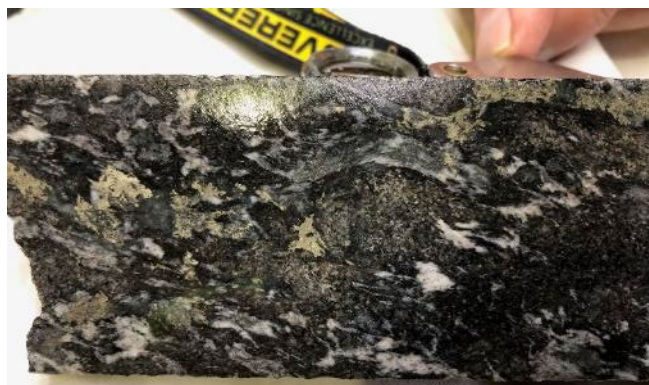
Figure 10 – core from 236m depth within PDD002 completed at the Paterson Project showing disseminated and semi-massive sulphide as void infill within strongly altered breccia.
