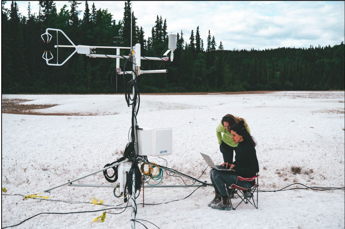
Figure 1: Arca scientists demonstrate how carbon dioxide mineralisation rates are measured on mine tailings. Photo: Taku River Tingit First Nation traditional territory, British Columbia, Canada
