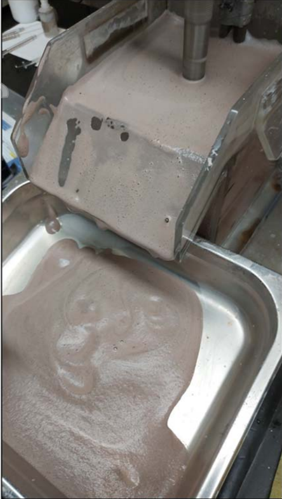
FIGURE 5: METALLURGICAL TESTING – FROTHER PRODUCT EXAMPLE
