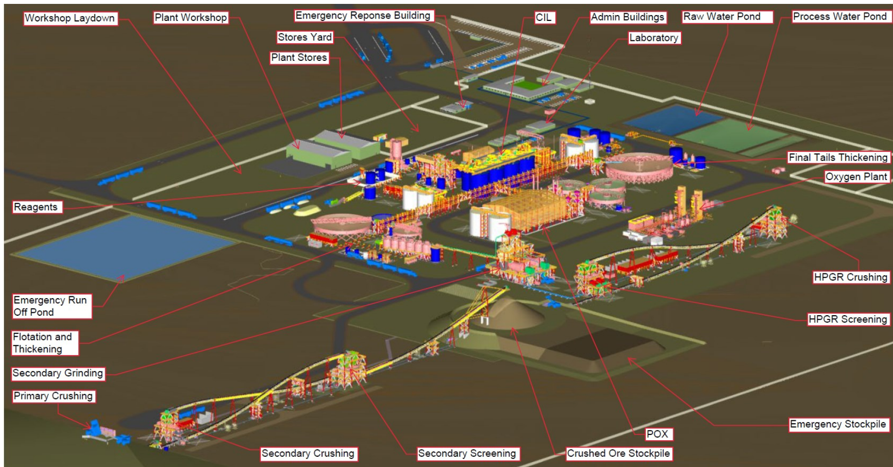
Figure 1-28: Process Plant Isometric
