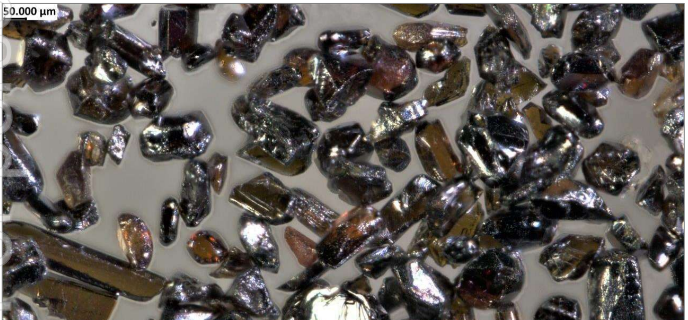
Figure 25: Photomicrograph of high purity rutile product
