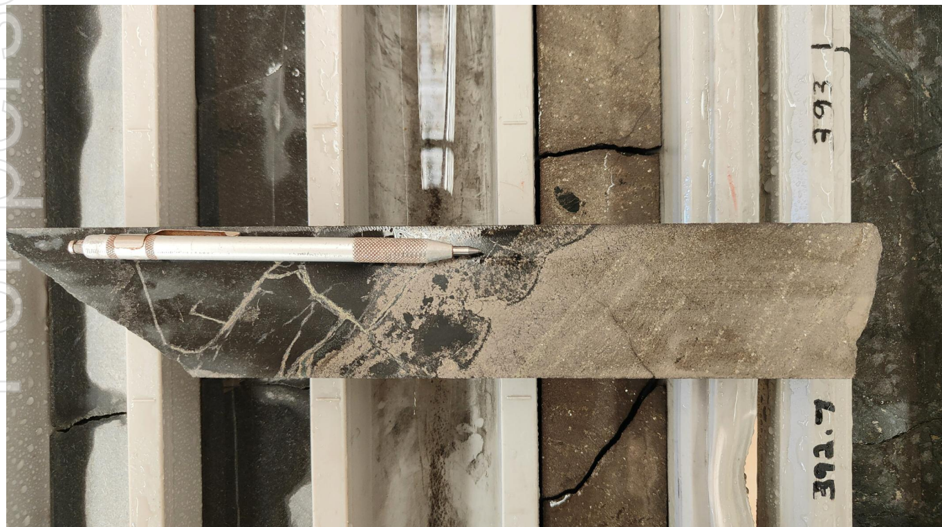
Photo above: Emu Lake Drillhole AELD0003 showing basal contact of massive sulphide intersection with footwall dacite. AELD0003: 2.72m at 5.42% Ni and 0.85% Cu from 391.04m including 1.23m at 8.22% Ni and 0.56% Cu from 391.04m (ARLASX 14 Jan 2022).
