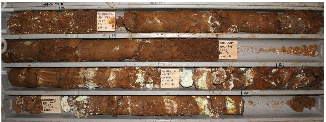
Photo above: Highway Drillhole AHID0012 showing Mineralised Neutraliser - comprised of goethite (brown) and magnesite saprock fragments (white).
