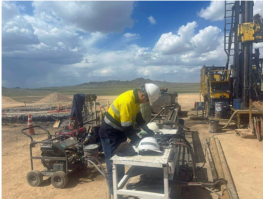
Excelsior Energy personnel operating Drill Stem Testing tools
