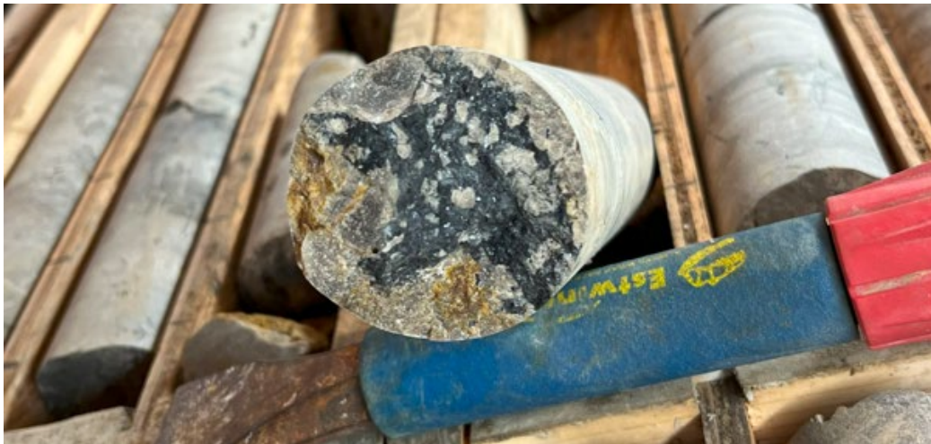
Figure 1: Drill core from diamond drill hole ST23-02 showing chalcocite (dark grey) copper sulphide breccia at approximately 354.7m downhole.
