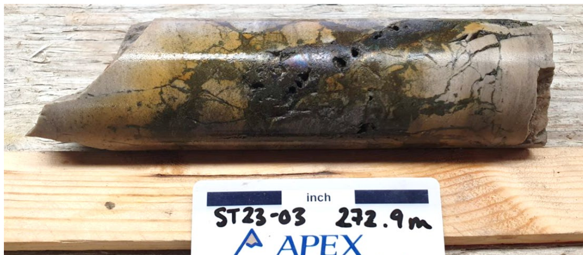
Figure 8: Breccia chalcocite (dark grey), bornite (purple/grey) and chalcopyrite (brassy) in drill hole ST23-03 from approximately 272.9m downhole.
