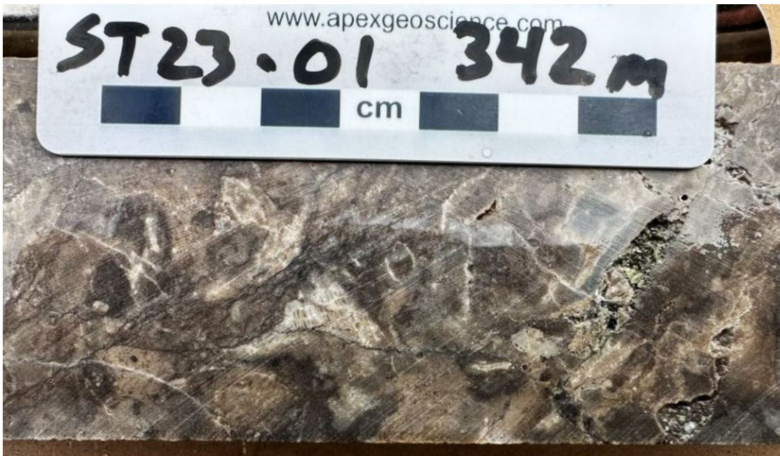
Figure 3: Chalcopyrite (brassy) in vugs and veinlets in drill hole ST23-01 from approximately 342m downhole.
