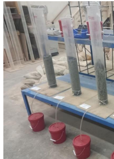
Figure 4b: Heap leaching simulated by top fed columns
