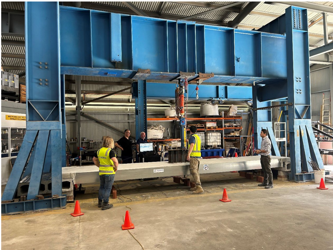
Image 3. Live Load performance testing
