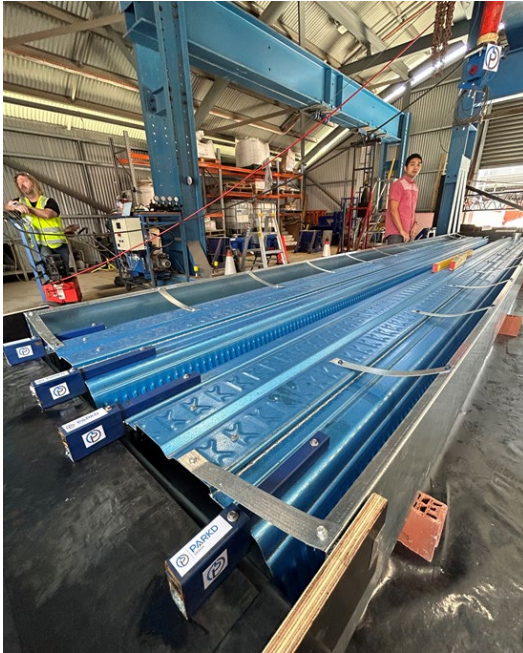
Image 1. Slab System test preparation
