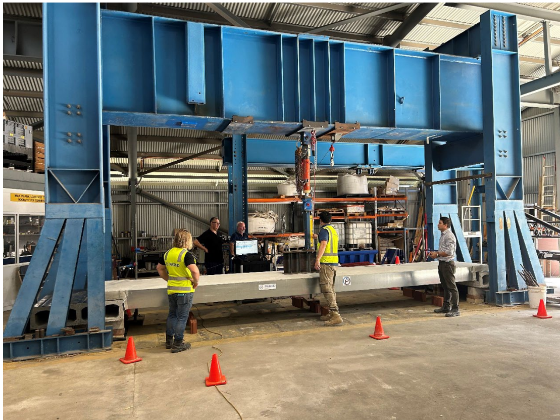
Image 3. Live Load performance testing
