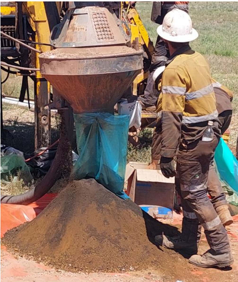
Figure 7 – Manganese mineralisation emerging from cyclone during drilling operations (JTRC288, 28m)
