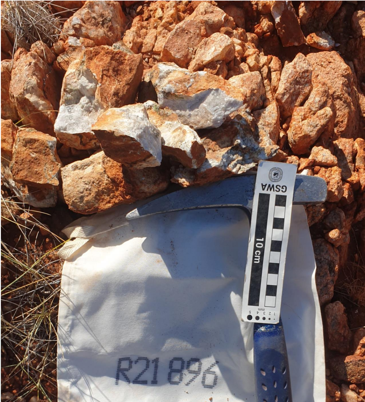
Figure 4: Rock sample R21896, collected from a 1.5-metre wide x 10m long pegmatite outcrop
