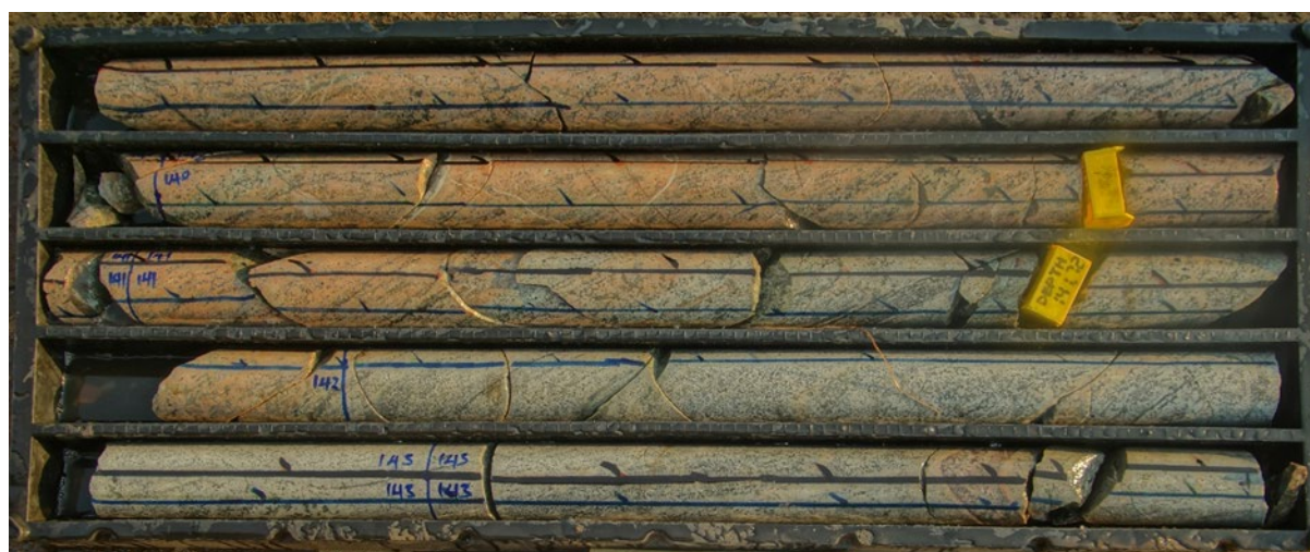
Figure 3. Diamond drill core from hole MDD 005 containing potential REE mineralisation from visual inspection (pinkish coral colour) from approximately 139m to 143m down hole, refer Table 2 for mineral estimates.
