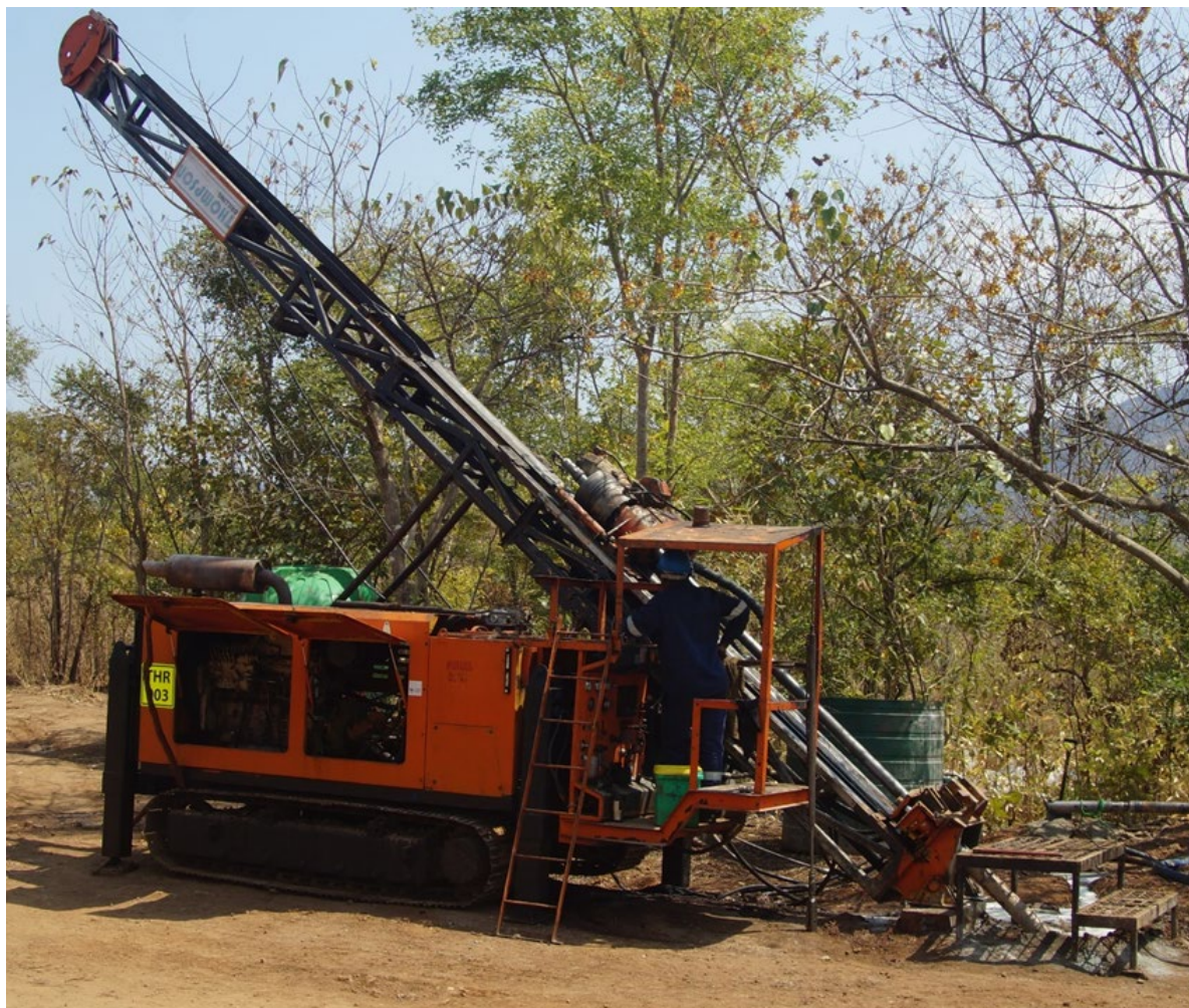
Figure 1. Diamond Drilling at Machinga North Prospect (MDD 005)
