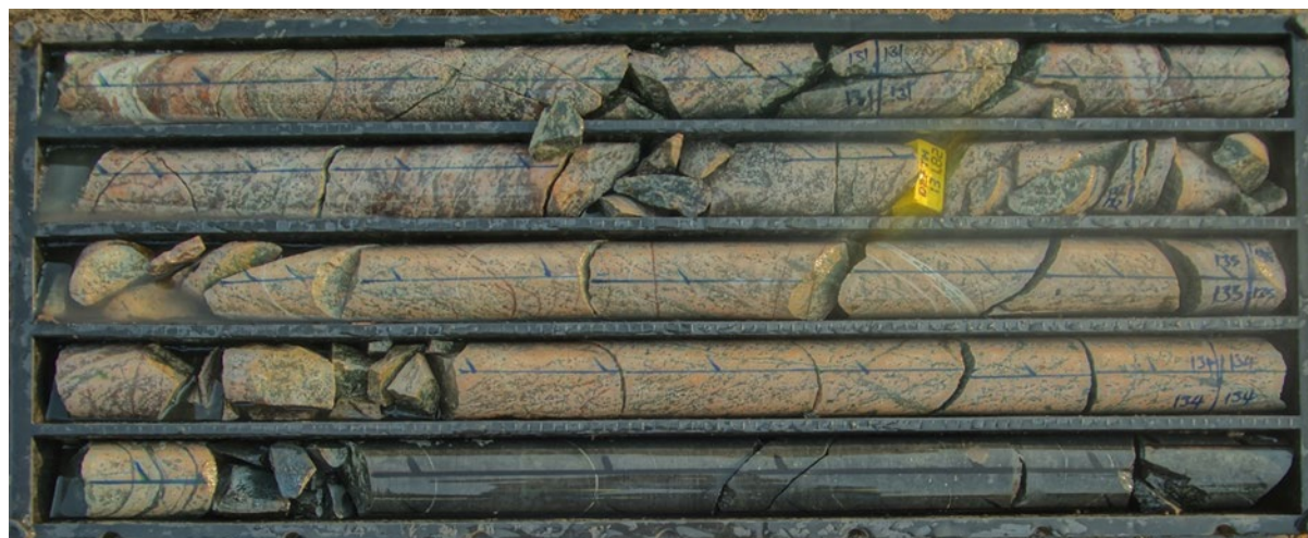
Figure 2. Diamond drill core from hole MDD 005 containing potential REE mineralisation from visual inspection (pinkish coral colour) from approximately 130m to 135m down hole, refer Table 2 for mineral estimates.
