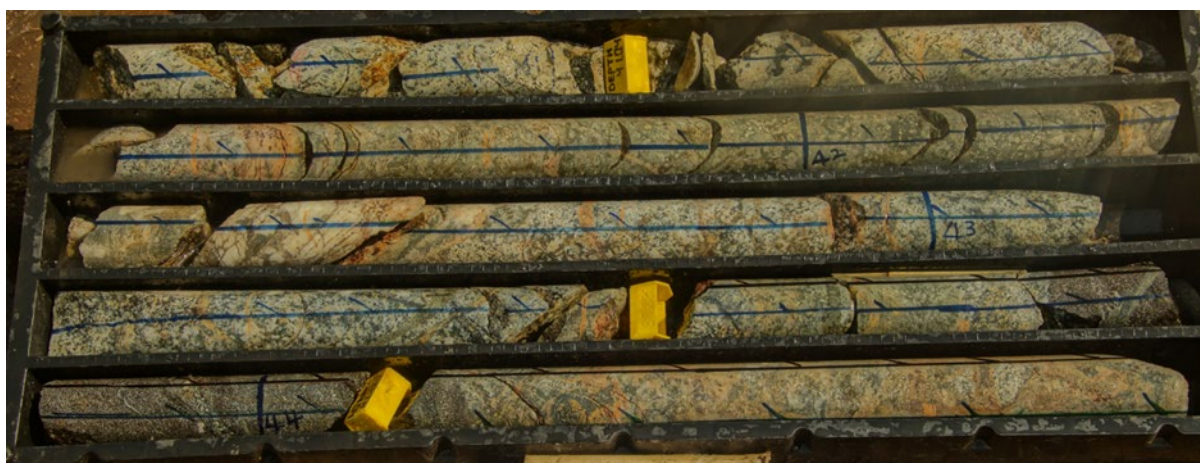
Figure 4. Diamond drill core from hole MDD 006 (metallurgical DD hole) containing potential REE mineralisation from visual inspection (pinkish coral colour) from approximately 41m to 45m down hole, refer to Table 2 for mineral estimates.
