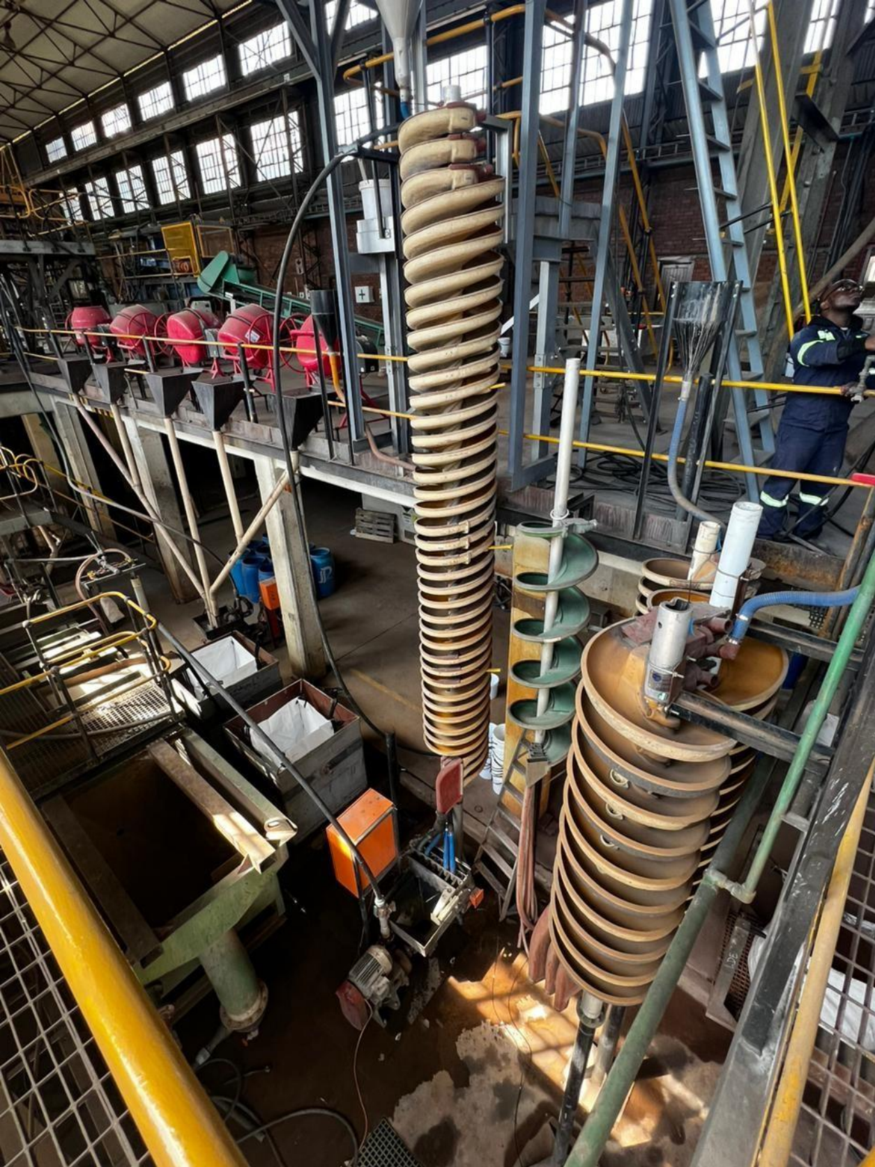
Image 1. Spiralling test-work being undertaken at LightDeepEarth in South Africa.
