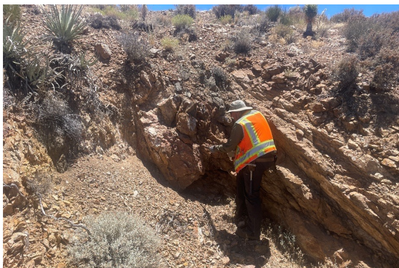
Figure 1: Historic Prospecting Pit Developed on mapped gossan in the south-east of El Campo Claims – US based team member Jim Baughman using a scintillometer to test the radiometric response.
