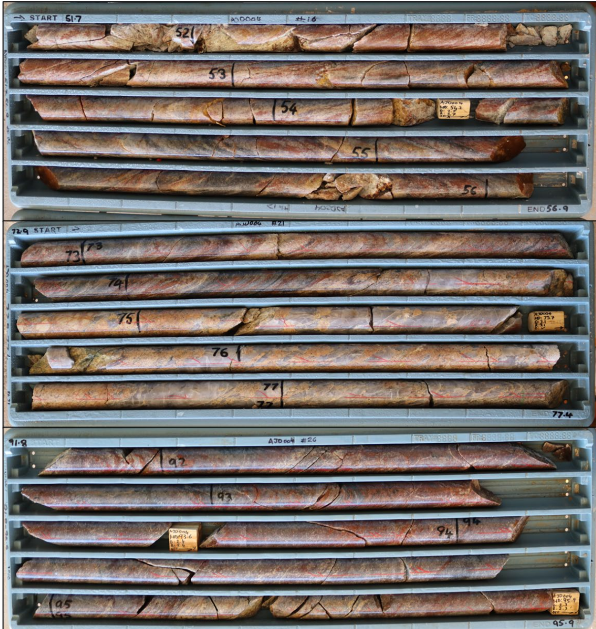
Figure 3: Core tray photos of AJDD004 at Catalina showing intense hematite alteration throughout sequence.
