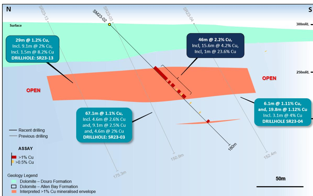
Figure 8: Geological section view at 465,015E showing drill hole SM23-02 details, the interpreted mineralisation envelopes (>1% Cu), and off-section previous drill holes on section 465050E.
