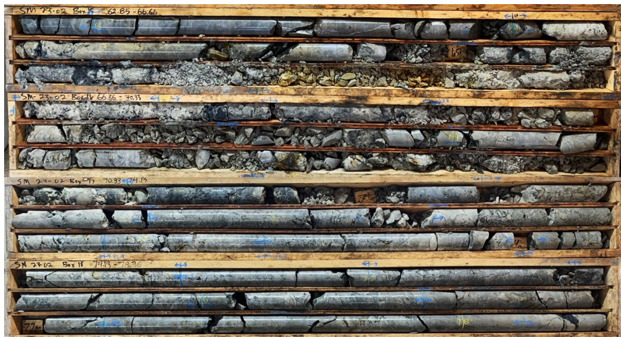
Figure 1: Drill core from resource diamond drill hole SM23-02 from the 4100N Zone showing chalcocite (dark grey) in dense brecciation, veining and faulting (now rubble). The interval is from approximately 62.85m to 78m downhole and contains an average grade of 6.4% Cu between 65m and 73.3m.
